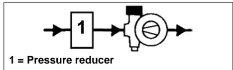
Fig. 2: Pressure reducer upstream of the unit
