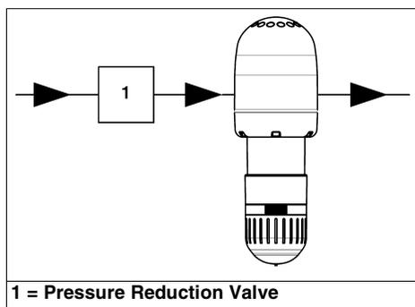
Fig. 2: Pressure Reduction Valve Fitted in Series in Front of the Jewel Water Device
