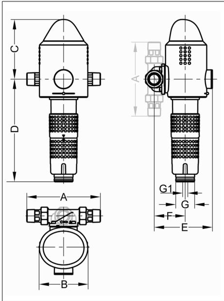
Fig. 7: Installation dimensions  $\frac{3}{4}$ " -  $1\frac{1}{4}$ "
