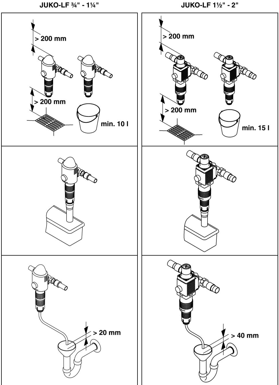
Fig. 5: Backwashing water discharge options
