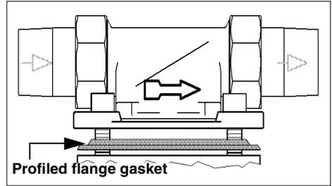
Fig. 8: Built-in rotary flange
