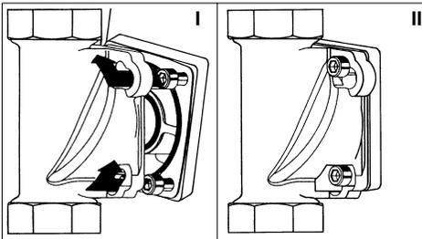
Fig. 7: Built-in rotary flange with bayonet fixture
