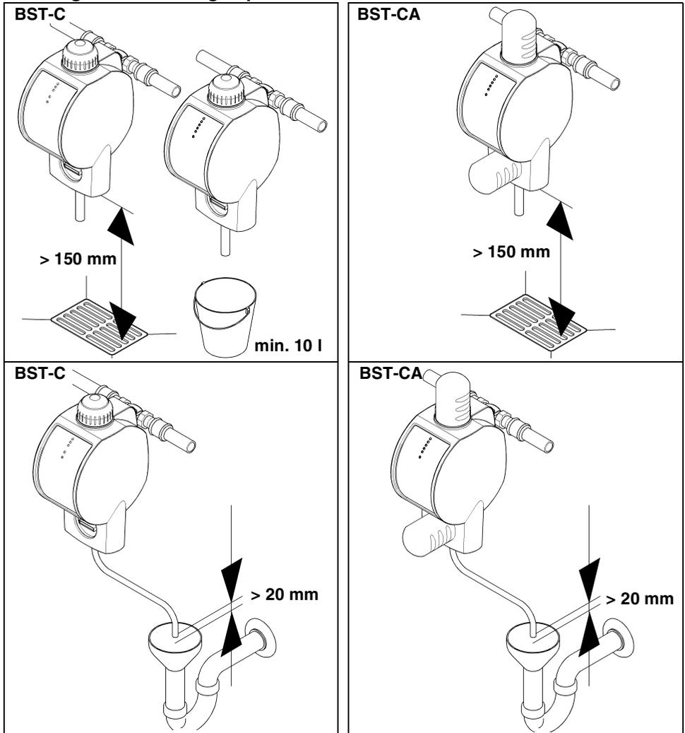
Fig. 9: Flushing water discharge options
