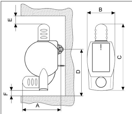
Fig. 13: Mounting Dimensions example BST-CA
