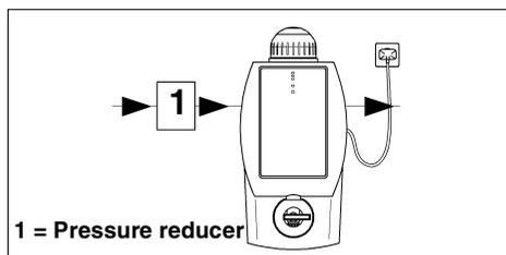
Fig. 2: Pressure reducer upstream of the water treatment device e.g. BST-C
