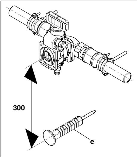
Fig. 6: Wall support with bypass valve
