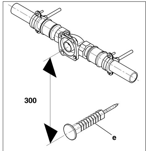
Fig. 5: Wall support without bypass valve
