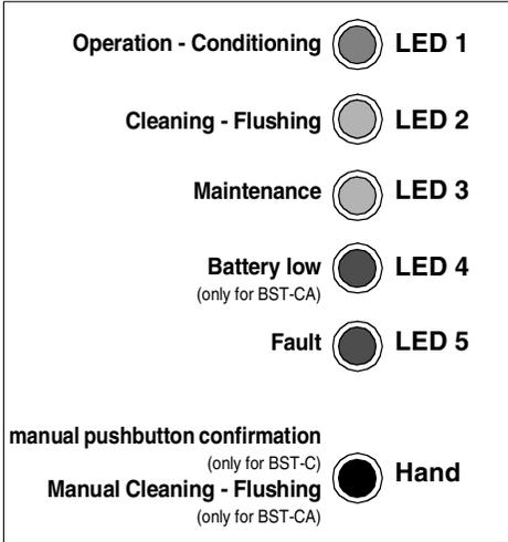
Fig. 12: Control lamps, manual pushbuttons
