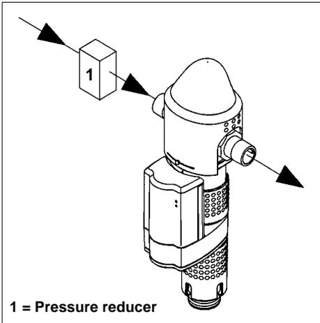
Fig. 2: Pressure reducer upstream of the unit
