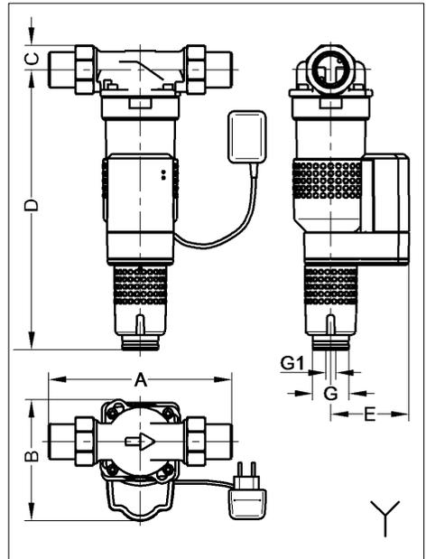
Fig. 15: Installation dimensions
