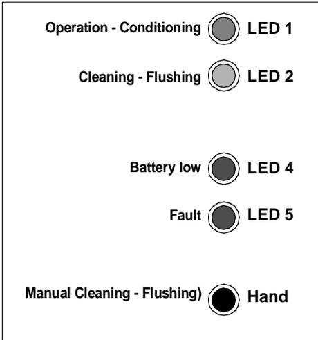
Fig. 11: Control lamps, manual pushbuttons
