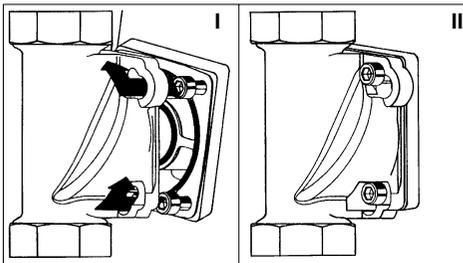
Fig. 5: Built-in rotary flange with bayonet fixture
