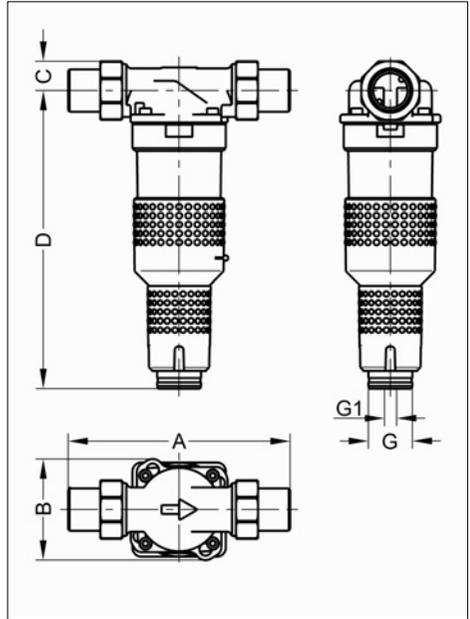
Fig. 8: Installation dimensions JSY-LF 1½" - 2"
