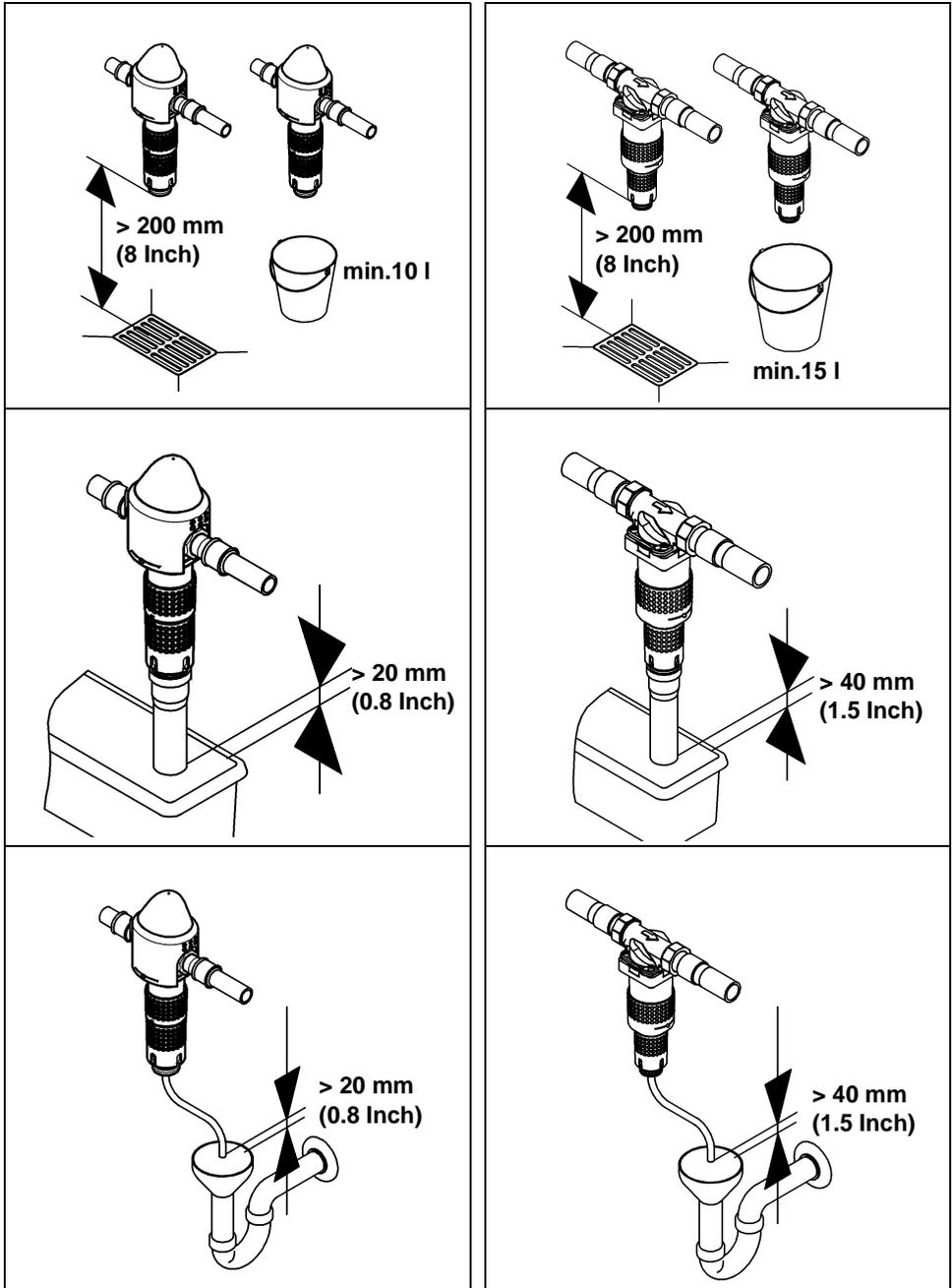
Abb. 5: Backwashing water discharge options
