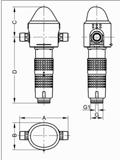
Fig. 7: Installation dimensions JSY-LF ¾" - 1¼"
